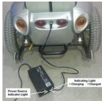
**Figure 22a Charger - Lead Acid Battery**
